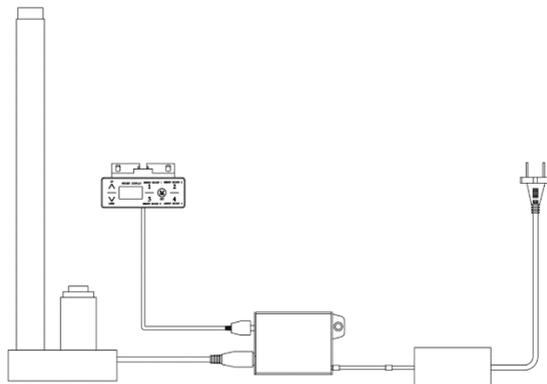
Connect the components as shown in the figure. Make sure that the connectors are firmly plugged in. Now connect the power cable, the display should show „72.0“ for a few seconds. This means that the table frame has been successfully wired.
